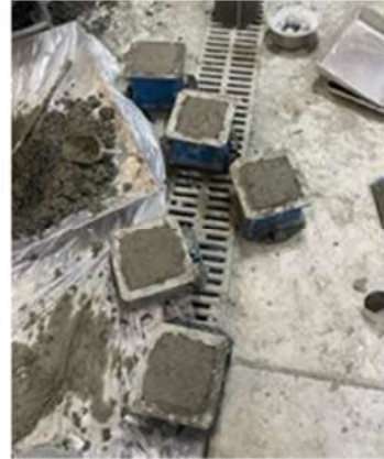
Fig 2.5 Casting of cubes
