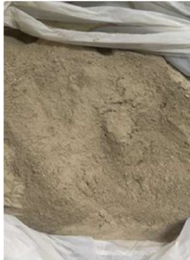
Fig 2.1 Sarooj used as a replacement for cement
