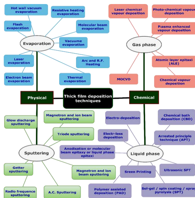
Figure 2. Different approaches for the deposition of thick film techniques
