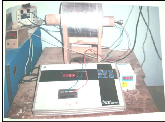
Fig. 4.3 Experimental setup for a. c./d. c resistivity
