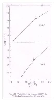
Using the above equation and the plots of logp versus reciprocal of temperature, the activation energy of all the samples has been calculated and the values were presented in Table 4.1.
