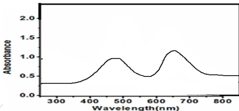
Fig.3 Electronic spectrum of  $[\text{Cu}(\text{cq})(\text{mq})\text{Cl}_2] \cdot 2\text{H}_2\text{O}$
