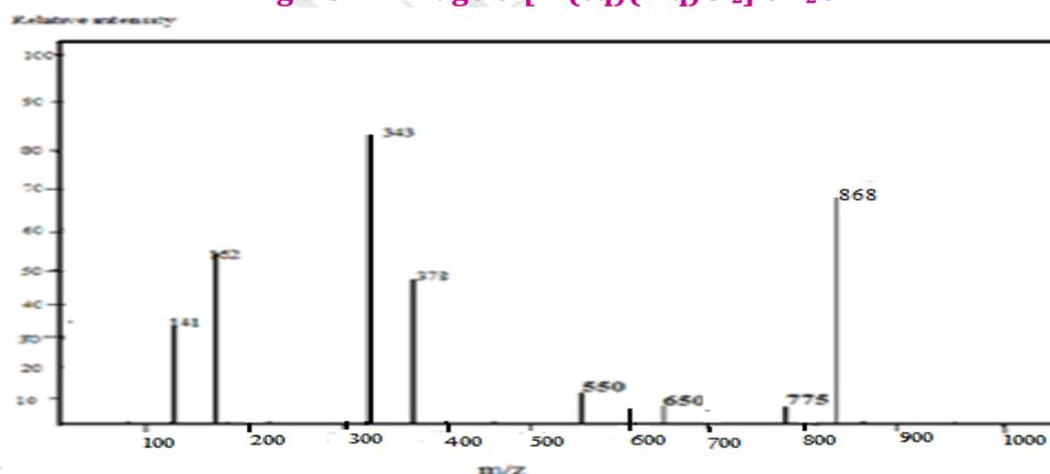
Fig.10 FAB Mass spectrum of  $[\text{Cu}(\text{cq})(\text{mq})\text{Cl}_2] \cdot 2\text{H}_2\text{O}$
