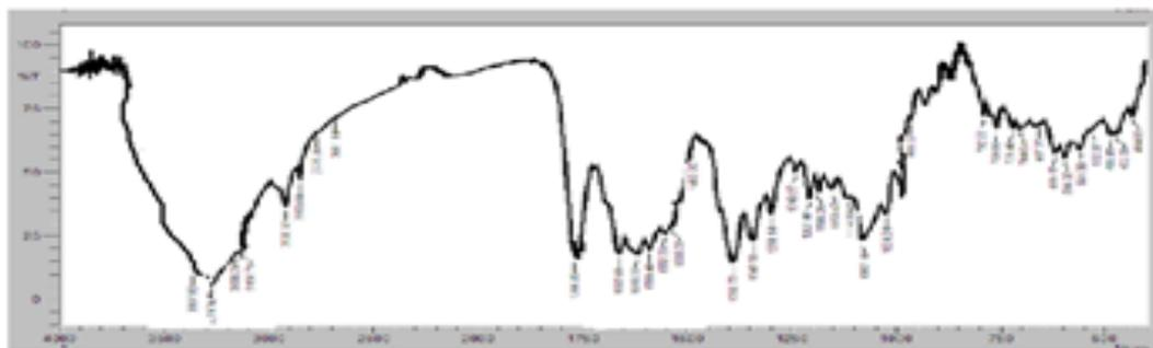
Wave number( $\text{cm}^{-1}$ )Fig 2 IR spectrum of  $[\text{Fe}(\text{cq})(\text{mq})(\text{H}_2\text{O})\text{Cl}_3] \cdot 5\text{H}_2\text{O}$
