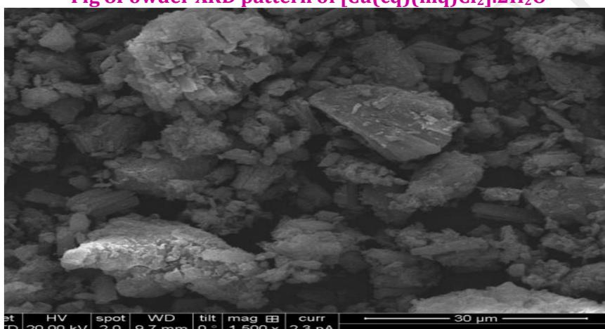
Fig 9 SEM image of  $[\text{Ni}(\text{cq})(\text{mq})\text{Cl}_2] \cdot 6\text{H}_2\text{O}$
