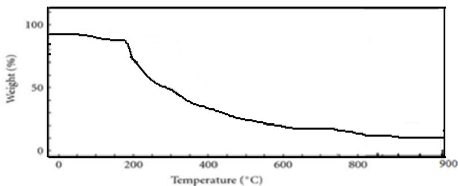
Fig.6 TGA pattern of  $[Cu(cq)(mq)Cl_2].2H_2O$
