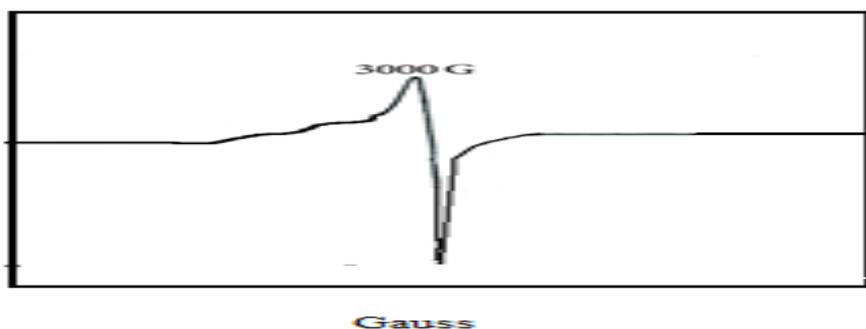
Fig.4 ESR spectrum of  $[Cu(cq)(mq)Cl_2].2H_2O$  at 300K
