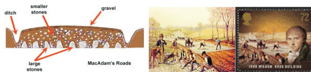
Figure 4 Macadam pavement construction
