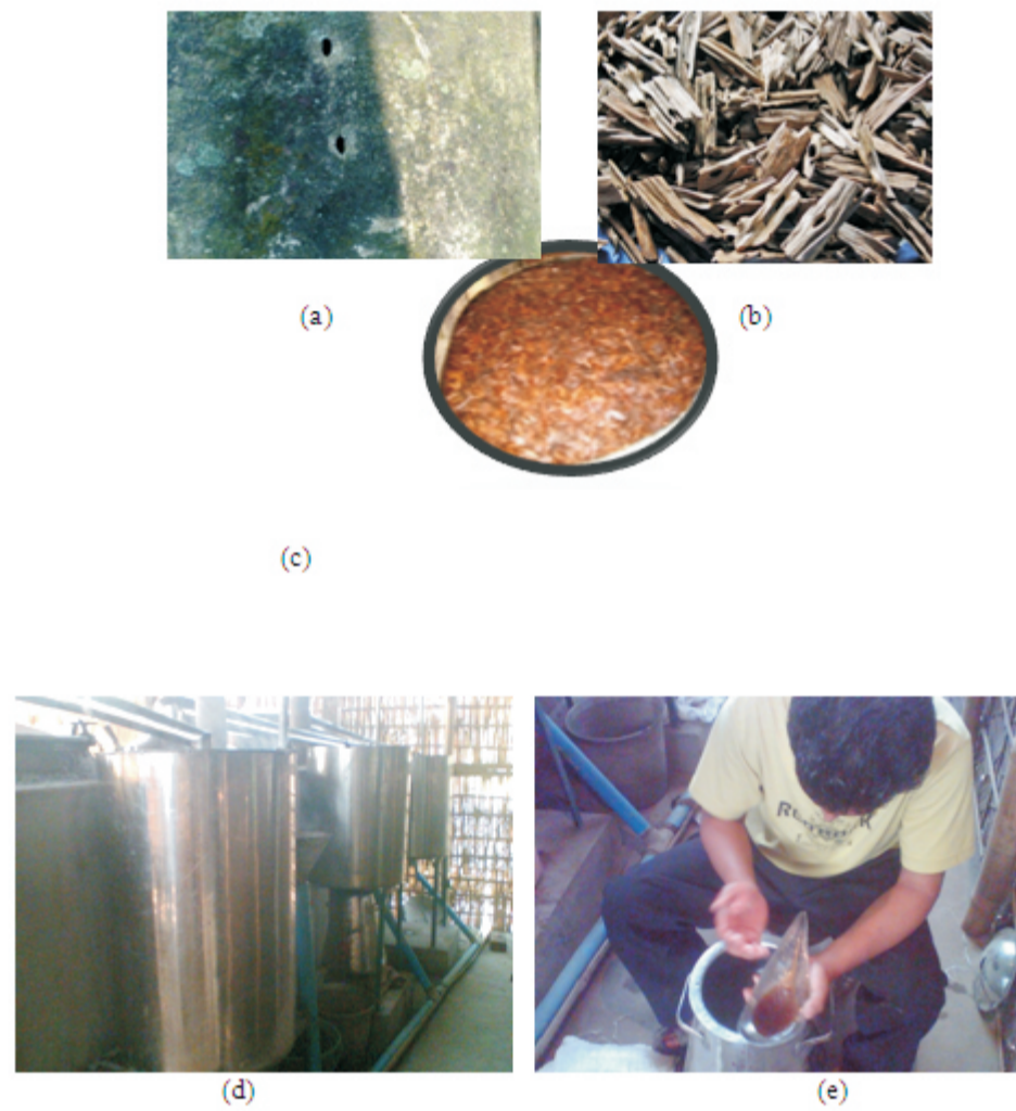
Fig. 5 Process of obtaining agar oil (a) Agarwood as in tree (b) Agarwood chips (c) Chips as in cooking chamber (d) Distillation unit and (e) Agar oil after distillation
