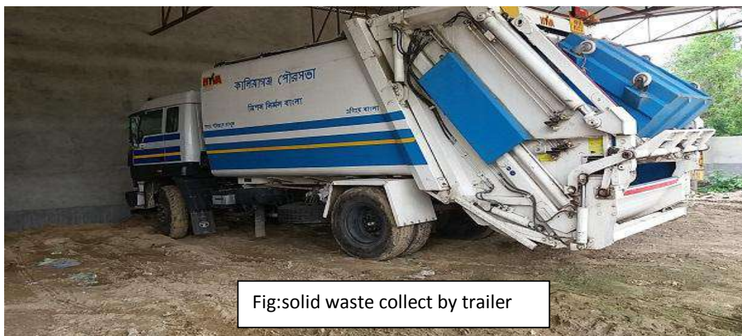
Fig:solid waste collect by compactor
