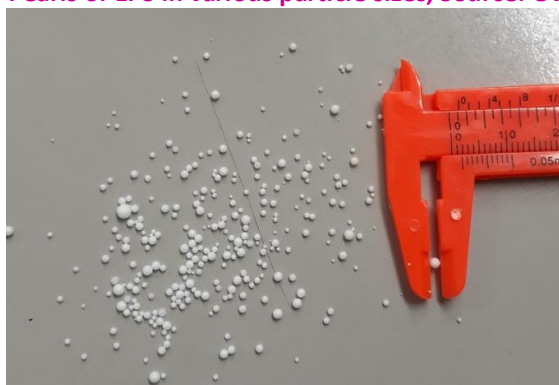
Figure 5 – Pearls of EPS in various particle sizes, Source: Own author.
