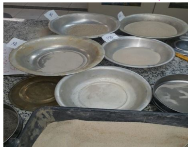
Figure4 – Sand divided into several fractions, Source: Own author.
