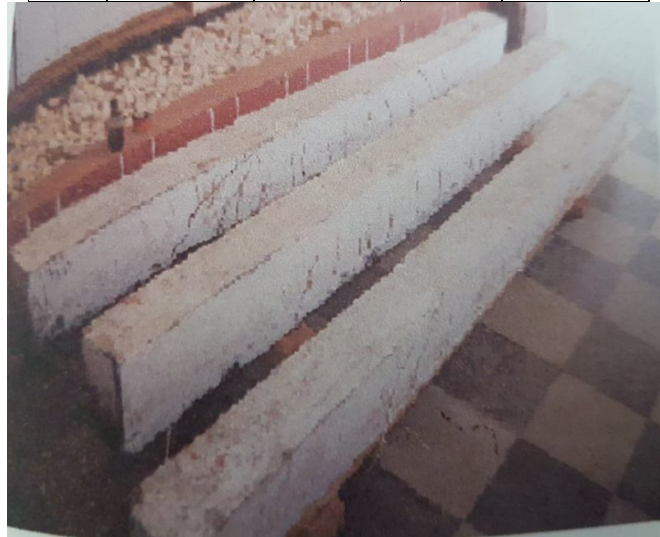
Fig 3 Beams after testing
