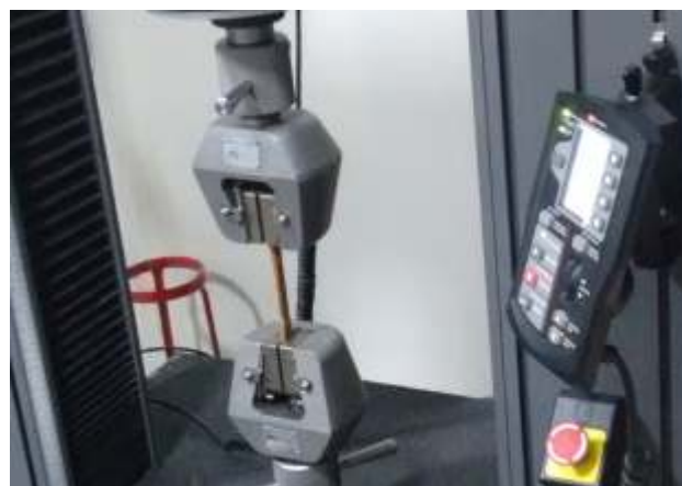
Figure 16: Electromechanical Universal Testing Machine mark INSTRON, model 5984 at the moment of starting the tensile force
