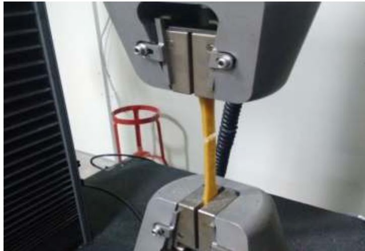
Figure 17: Electromechanical Universal Testing Machine Mark INSTRON, Model 5984 at the time when the test body fails
