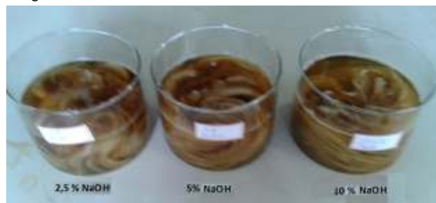
Figure 4: Chemical treatment of the fibers with sodium hydroxide
