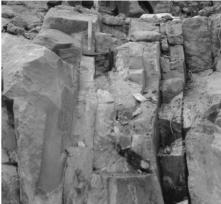
Figure 4a: Intense steep N-S fracturing with dip >85°E. Location: Agrewadi – 73°30'31"E; 16°40'20"N
