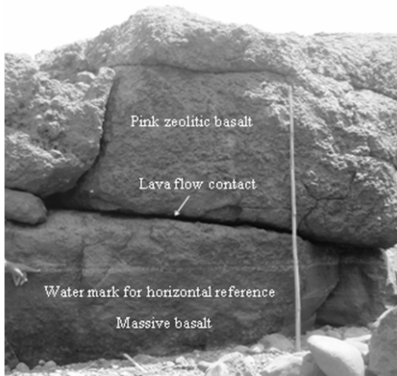
Figure 4b: 60° tilt of lava flow contact towards east. Location Daphlewadi – 73°41'36"E; 16°56'56"N
