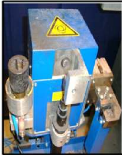
Figure 7: torch cleaning station.
