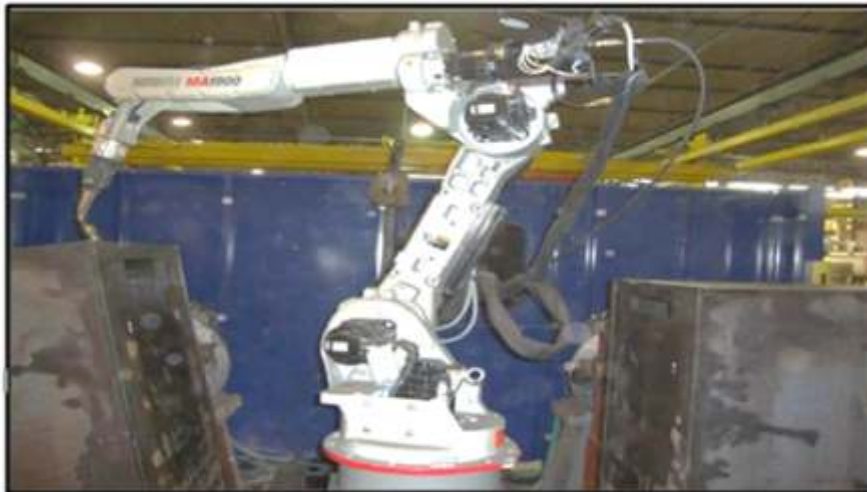
Figure 3: Robot welding process used in MIG / MAG
