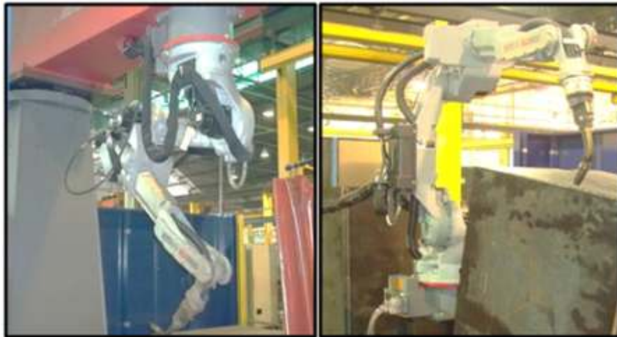
Figure 4: Welding Robot parts, and closing respectively.
