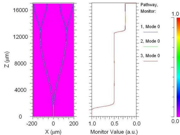
Fig. 3.3 show the designed  $1 \times 4$  optical power splitter and its performance. In all Y- branching arms, cosine S-bends were used to minimize the radiation losses at the splitting junction. The splitting ratio of a Y-branch waveguide depends only on the symmetry and is a wavelength independent 3-dB splitter. The port separation at the output has been standardized to  $127 \mu\text{m}$  (center-to-center) so as to match standard fibre ribbon for pigtailling.
