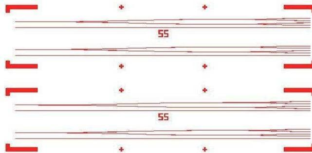
The mask was fabricated by direct-write technique through Laser Pattern Generator (Heidelberg Instruments, Germany) at the Mask Fabrication Facility in CSIR-CEERI, Pilani. The fabricated mask was observed under the microscope to look for defective areas such as pin holes and any other unwanted features.
