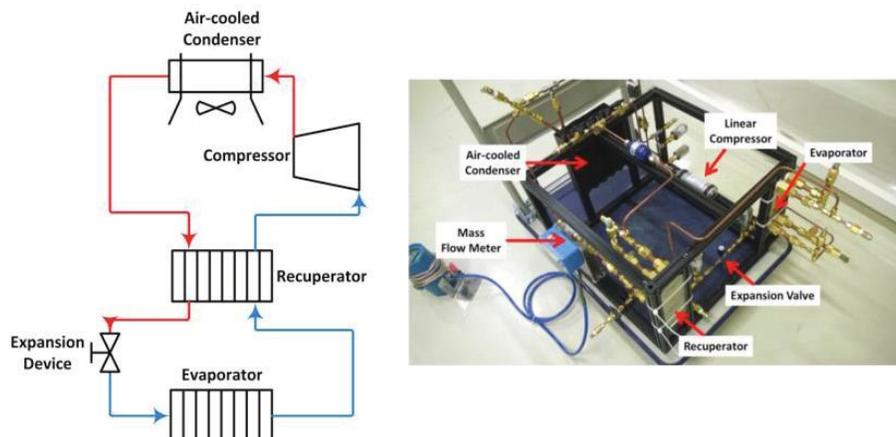
**Fig. 1. Schematic diagram of VCC test-bed setup (left) and prototype photo before insulation (right)**
