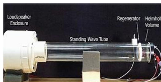
Figure.1. Thermo-acoustic refrigerator setup
