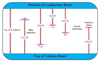
Al-ZnO thin film, electrons contributing from oxygen ions showed an increase in  $PO_2$ . The photoluminescence (PL) spectra of the films show the emission peaks visible from the faulty state. The optical properties of thin films confirm their applicability to optoelectronic devices. Room temperature, current-voltage (I-V) plot shows low resistivity in thin films  $\sim 10-2$  ( $\Omega$ -cm).
