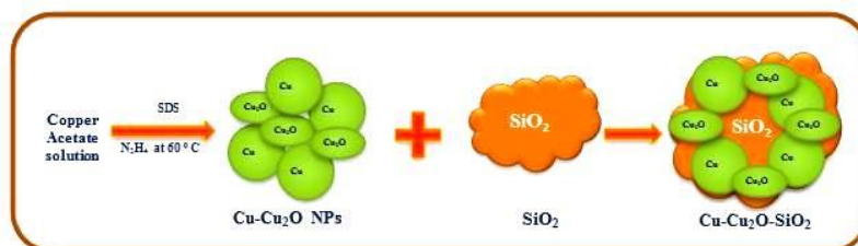
Fig. 1.1: Synthetic route of Cu–Cu 2 O–SiO 2 nanocomposites.
