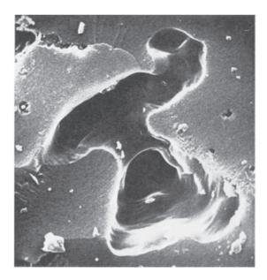
Fig. 1 Pores of n Pt/CMS catalyst ( x 6400). Large pore diameter approx. 3p. Small pore diameter approx. 0.5~.
